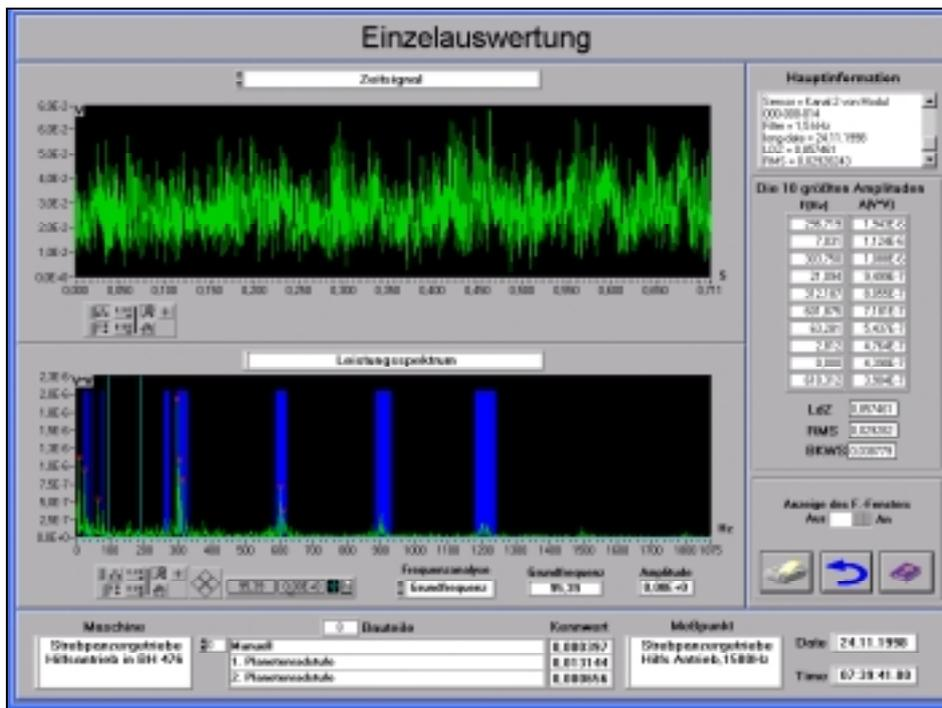
**Figure 4: Online-machine diagnosis (DIAMIS) data of a chain-conveyor drive**
