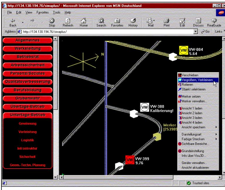
**Figure 3 : Visualization of online-ventilation-data within an intranet environment, WEB-based**
