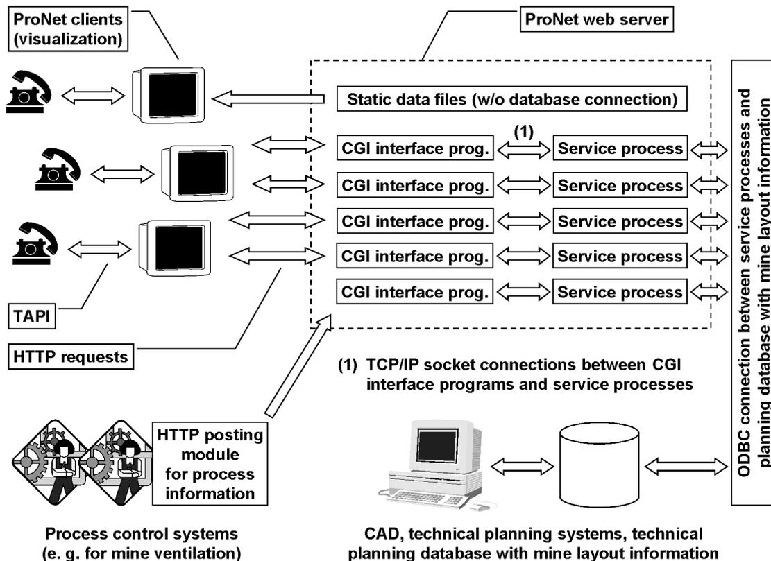
Figure 3. Internal structure and flow of information.
