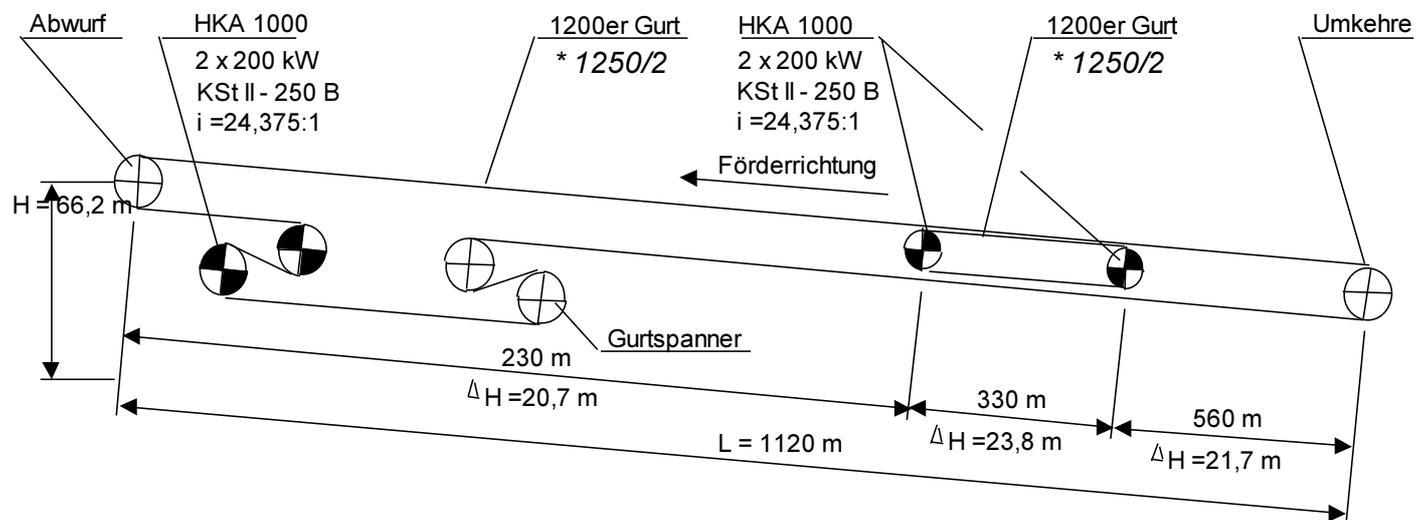
Figure 2: example of standardized document: layout of belt-conveyor on German hard coal mine
