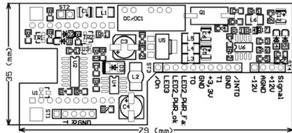
Figure 2. PCB Layout of the wireless sensor
