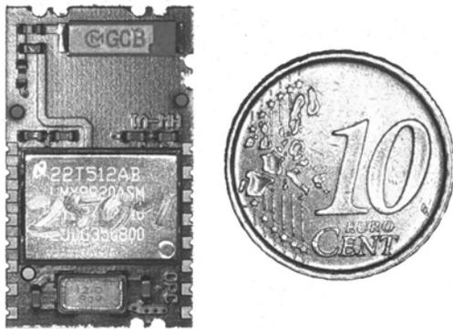
Figure 1. The Amber Wireless Bluetooth module with integrated ceramic antenna (top)
